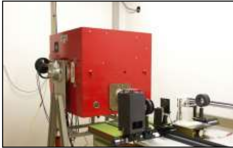
Institut Curie: Kinetron Mean Dose Rate: 0.01 - 7500 Gy/s
