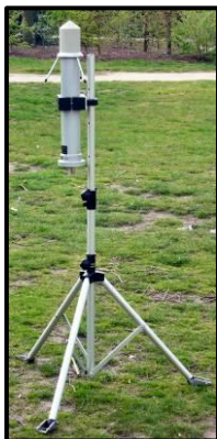
Figure 7. Illustration of a mobile station for measuring the dose rate (ambient gamma radioactivity).
