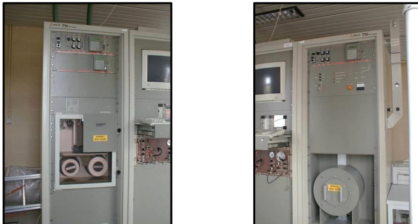
Figure 4. (Left) Illustration of an alpha/beta unit of measure with a view of the pull-down filter tape that collects dust and particles from the air. (Right) The radioactive iodine detector in its shielding (cylinder) and the parallelepiped tube containing the active carbon cartridges (on the right side).
