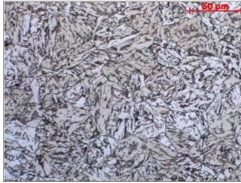
Figure 5.8: VB395/6BF: light zone microstructure: upper bainite (red scale 50 \mu\text{m} ).
