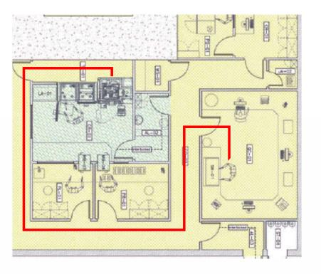
Transport of quality control sample in shielded container from hotcell drawer system to QC-lab
